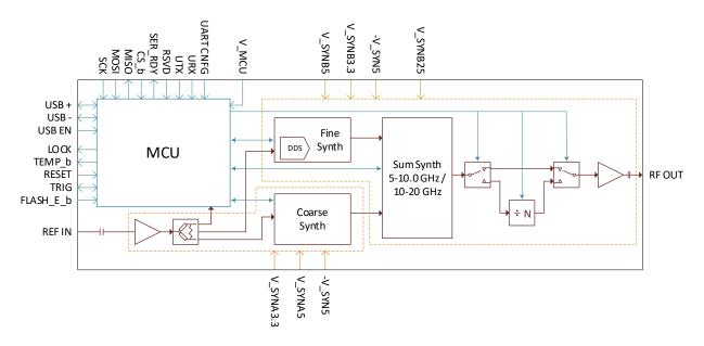
Figure 2. Block Diagram of the SC801A/SC802A
