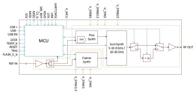
Figure 1. SC801A / SC802A Functional Block Diagram
