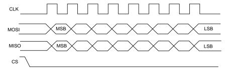
Figure 3. SPI Mode 1 shown.
