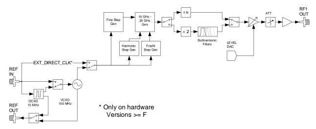
Figure 2. UHFS block diagram
