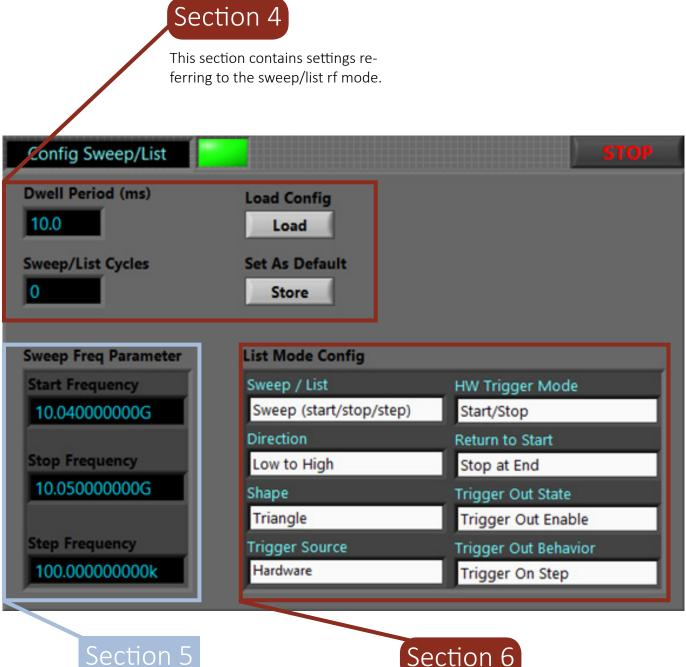
The Sweep Frequency Parameter section contains the start, stop, and step inputs for controlling the list sweep parameters.
