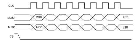
Figure 3. SPI Mode - Data clocked in on falling clock edge.
