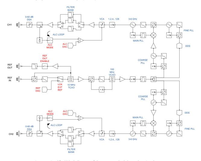
Figure 2. Simplified block diagram of the SC5506A dual channel RF signal source.
