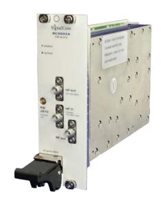
Frequency accuracy is provided by an onboard 10 MHz temperature compensated crystal oscillator (TCXO) which can be phase locked to an external reference source if required, and it is recommended to do so in applications that may require a more stable and accurate base reference.
