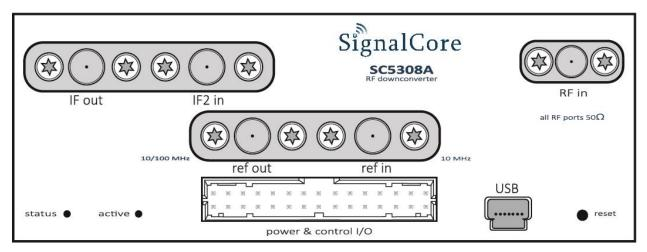
The SC5308A is a serial controlled core module with front face connections shown below:
