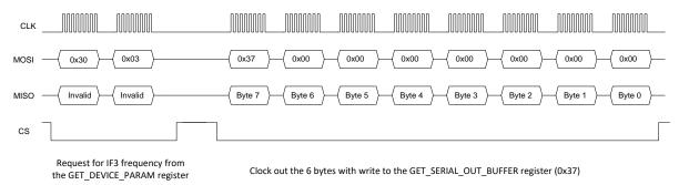
Figure 11. Query example: Write followed by Read to the GET\_SERIAL\_BUFFER
