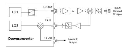
Figure 6. Application example of using external LO1 for down conversion of a Ka band signal.
