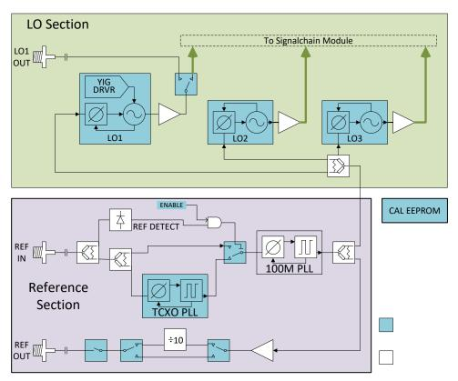
Figure 5. Block diagram of the local oscillator.
