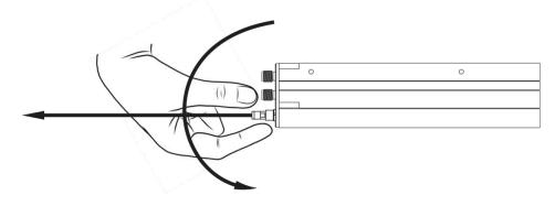
Figure 2. Proper Removal of Latching-Style Ribbon Cable Connectors
